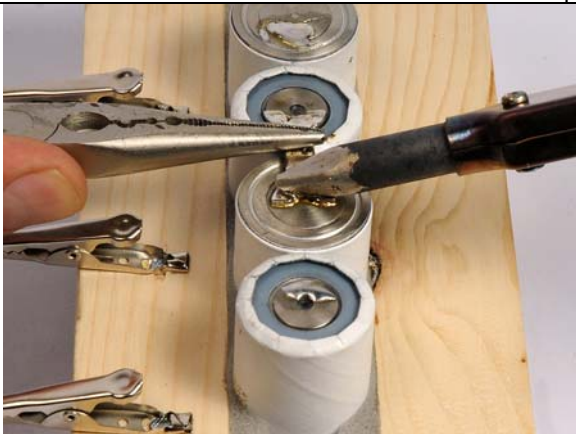
Be sure to use a HOT iron and apply bars and wires to cells within 2~3 seconds
