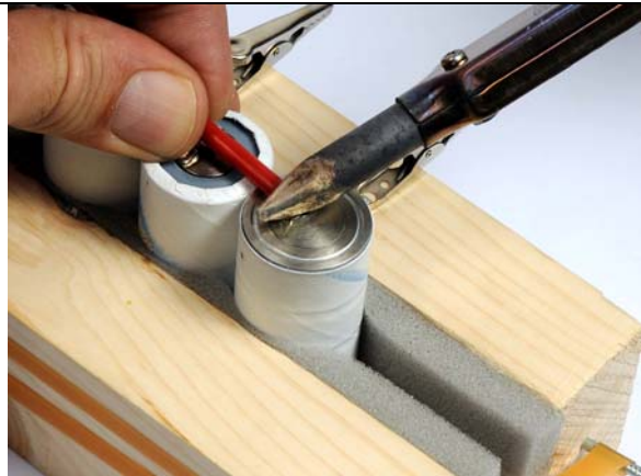
Be sure to use a HOT iron and apply bars and wires to cells within 2~3 seconds
