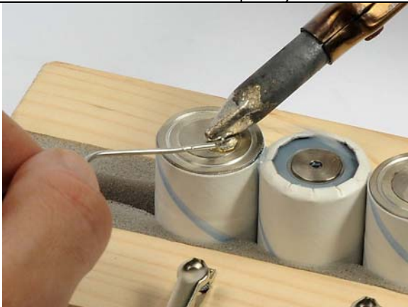
Tin the silicone output wires
