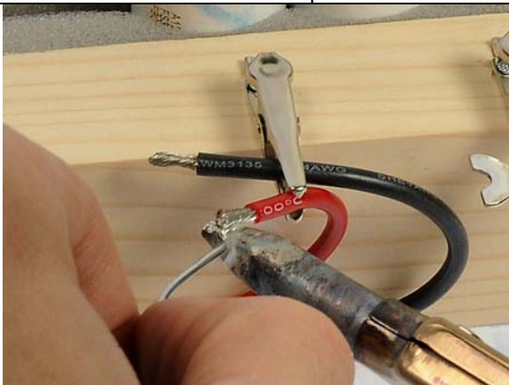
Be sure to use a HOT iron and apply bars and wires to cells within 2~3 seconds
